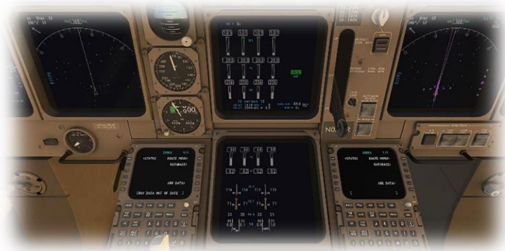
Engine-indicating and crew-alerting system (EICAS)
