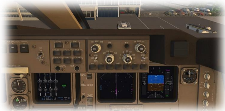
Co-Pilot's EFIS (Electronic Flight Instrument System) Control Panel
