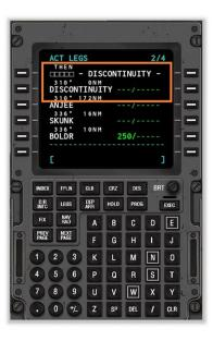
To repair the discontinuity, the missing waypoints BSR and CARME must be reintroduced into our flight plan, at the correct locations.
