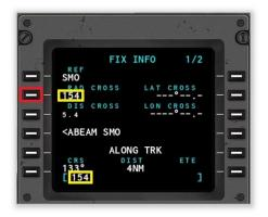
Input the desired radial (154) into the scratch pad.
