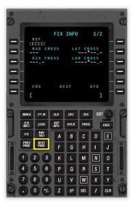
Input the name of the navigation aid that defines the fix. This is the Woodside VOR, which has the identifier OSI.
