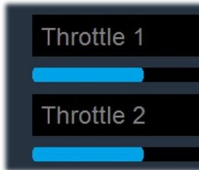
The King Air C90B is equipped with dual throttles – which control the torque (power) transmitted by the left and right engines. The throttles do not change the propeller RPM, which is set elsewhere, using the Prop Levers.
