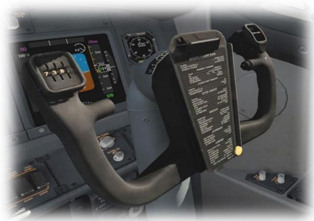
The Yoke / Stick / Joystick is operated by assigning a peripheral device to the "roll" and "pitch" axes in X-Plane. This is discussed in greater detail later in the guide.
