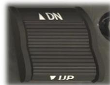
The Vertical Control can be used in this mode to change the IAS reference in 1 knot increments, either UP, or DOWN.
