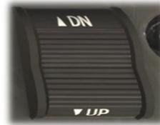
The Vertical Control can be used in this mode to change the VS in 200ft/minute increments, either UP, or DOWN.
