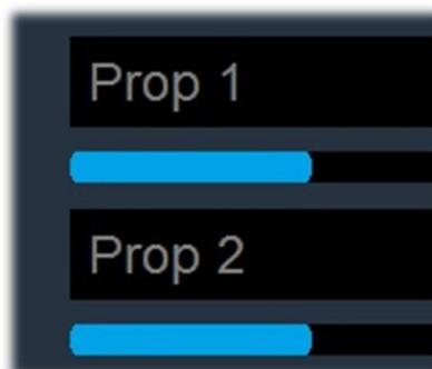
The King Air C90B is equipped with constant speed (and variable pitch) propellers. The RPM for each engine is controlled by a “governor”, and the desired RPM setting is made using the Prop Levers, which are part of the aircraft’s throttle quadrant. Once the RPM has been set, this remains the same, irrespective of the throttle position.
