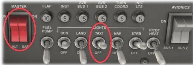
Toggle and Rocker switches are operated with a single click of the mouse. Place the mouse pointer slightly above, or below, the center point of the switch, depending on the direction you intend to move it. A small white arrow is displayed to confirm the intended direction. Click the mouse button to complete the operation.
