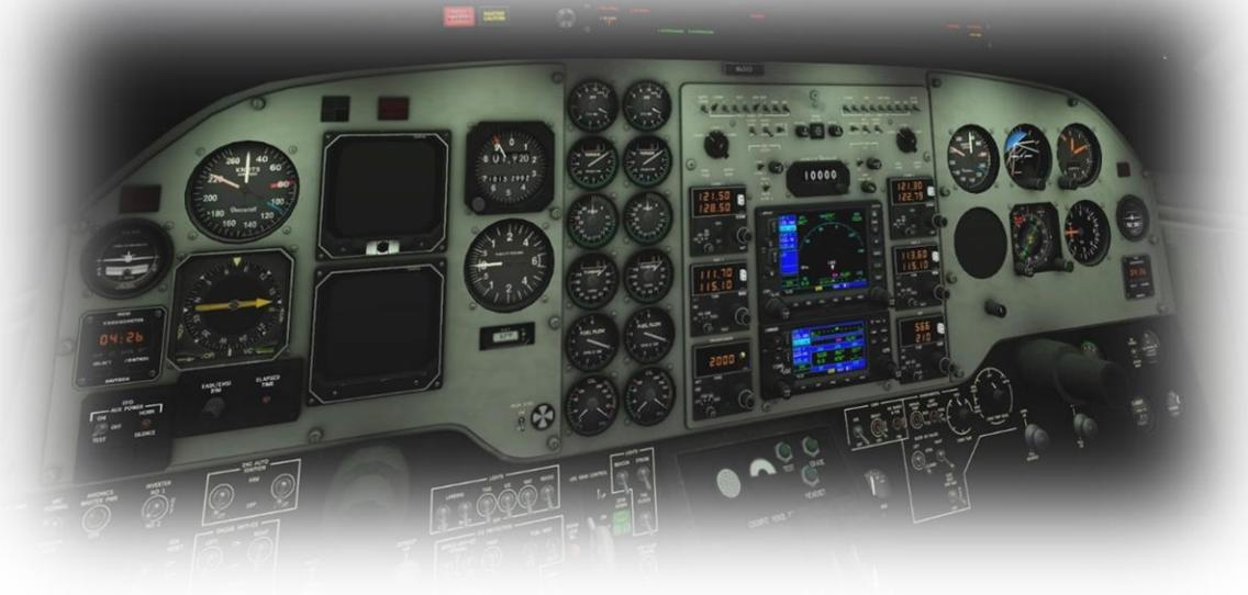
The X-Plane King Air C90B features a detailed 3-D cockpit with a great many of the primary controls and systems modeled, including: Flight controls (yoke, rudder pedals, throttles, prop levers, condition levers), electrical systems, navigation aids, radios, autopilot, instrument and cabin lighting, fuel and environmental systems.
