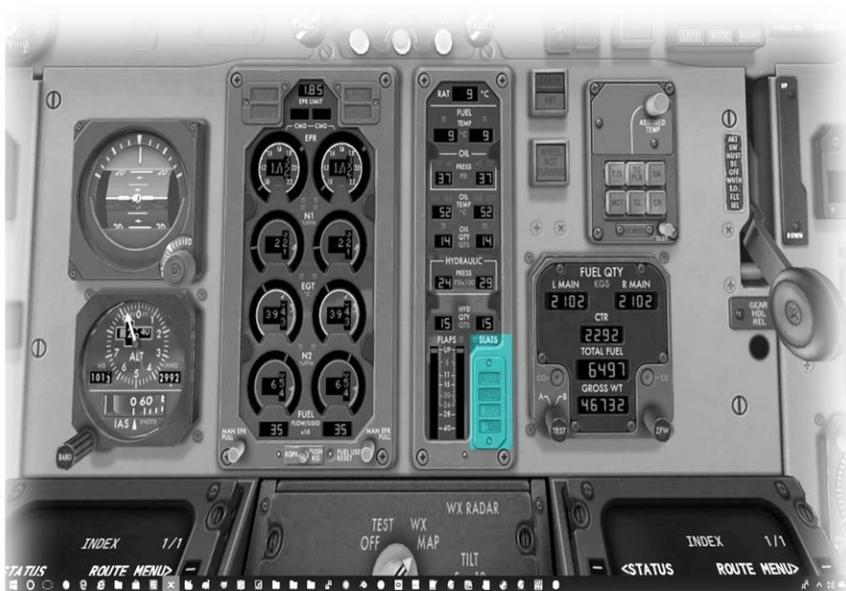
Slats are leading edge flaps that allow the wing to operate at a higher angle of attack. The MD-82 slats move in unison with the flaps and are operated with the same (flap) lever.
