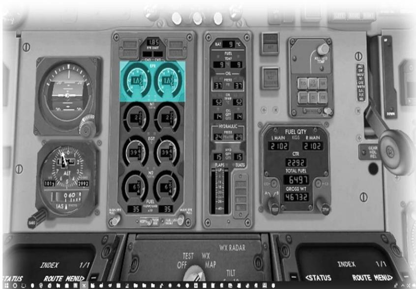
**[From Wikipedia]** The engine pressure ratio (EPR) is the total pressure ratio across a jet engine, measured as the ratio of the total pressure at the exit of the propelling nozzle divided by the total pressure at the entry to the compressor.
