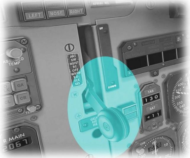
A close-up photograph of the cockpit's landing gear selector lever. The lever is a red, T-shaped handle mounted on a black base. It is positioned in the center of the lever's travel. The surrounding cockpit panel includes various controls and displays, such as the 'LEFT NOSE RIGHT' labels and the 'AIR TEMP' gauge. |
