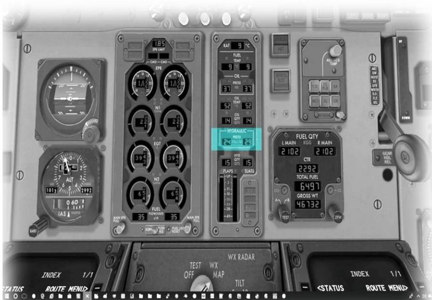
Left and right engine hydraulic pump pressure respectively.
