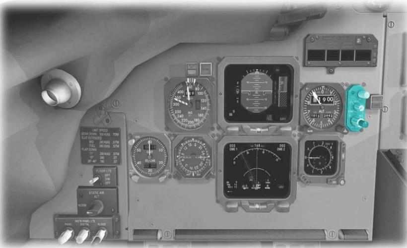
The rotary controls on this panel control the brightness of the EADI and EHSI displays.
