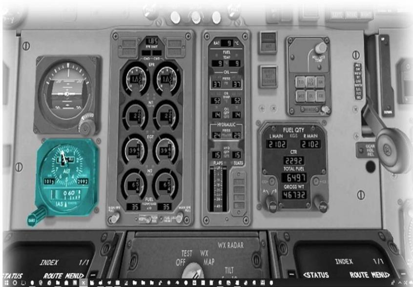
The backup Altimeter/Airspeed indicator in the real aircraft is powered by the pitot-static system, to provide redundancy, in case of failure of the primary instruments.
