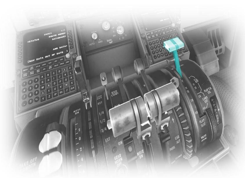
The Flap Lever operates the wing flaps. Wing flaps change the contour of the wing. When extended, the flaps generate more lift, and more drag, which is beneficial during the takeoff and the landing phases of the flight.
