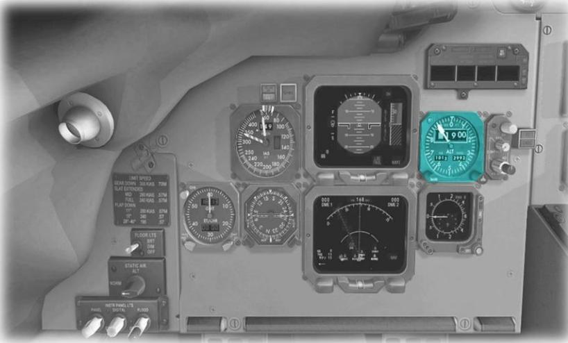
This instrument displays the altitude above sea level (not the ground). This model combines a digital and analog presentation.
