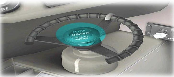
Large aircraft are frequently equipped with a tiller for nosewheel steering. The tiller here will respond to rudder commands for steering on the ground.
