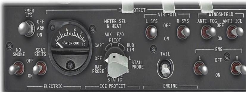
This panel monitors and controls the anti-icing systems.
