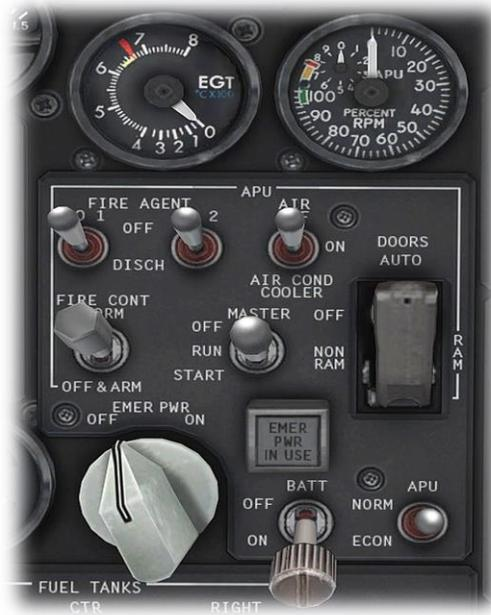
This panel contains the battery master switch that provides electrical power to the aircraft from the on-board batteries. Battery power provides a short-term electrical source, until a more sustainable source is activated.
