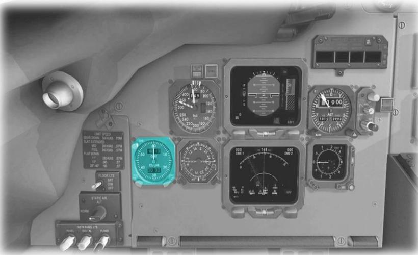
This instrument displays the current time, and (flight) elapsed time.
