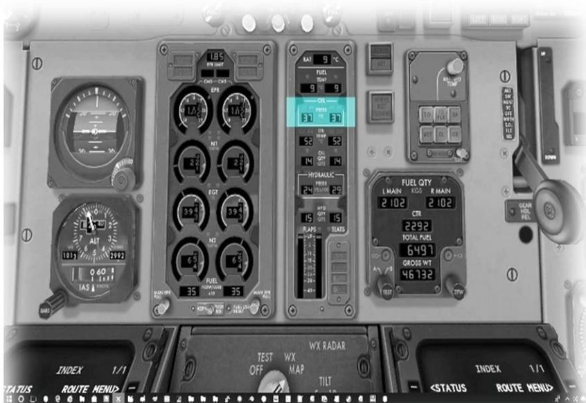
This is the left and right engine oil pressure respectively.
