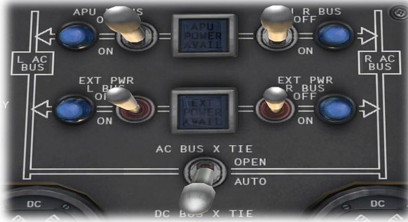
This panel is used to control the electrical power to the aircraft, when the main engines are not running.
