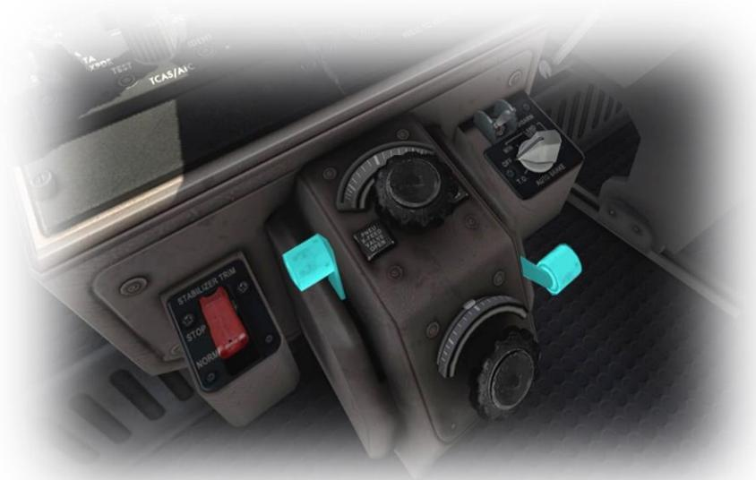
These levers are used to route pneumatic (air) pressure from the APU, GPU, or engine bleeds.
