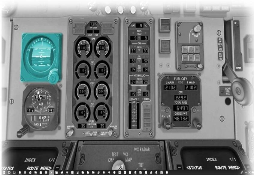
The backup Attitude Indicator is electrically powered and connected to bus zero. This provides redundancy, in case of failure of the primary instruments.
