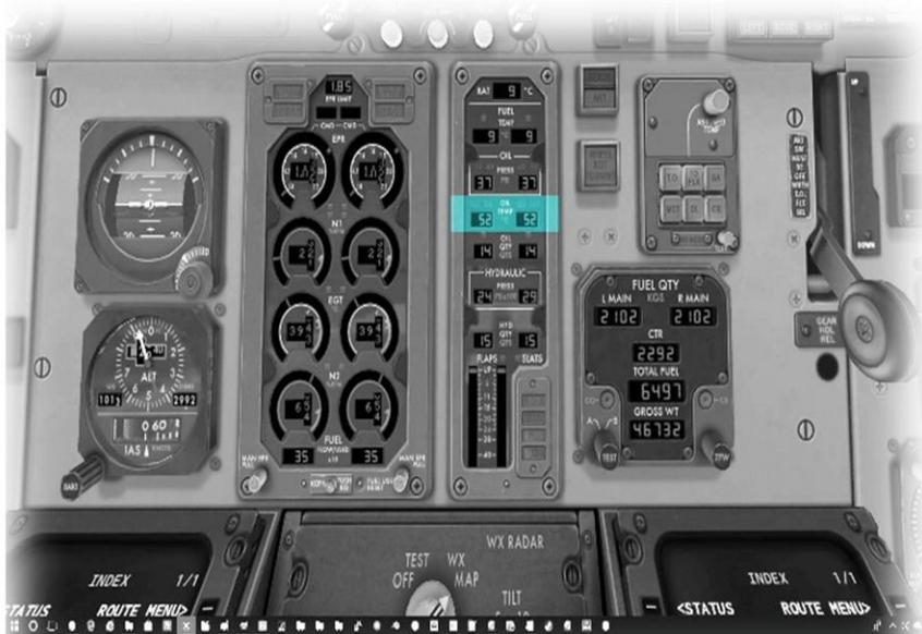
Left and right engine oil temperature respectively.
