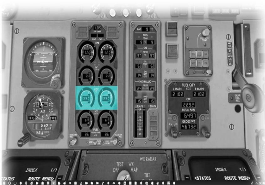
Exhaust gas temperature for the left and right engines respectively, in degrees Celsius.
