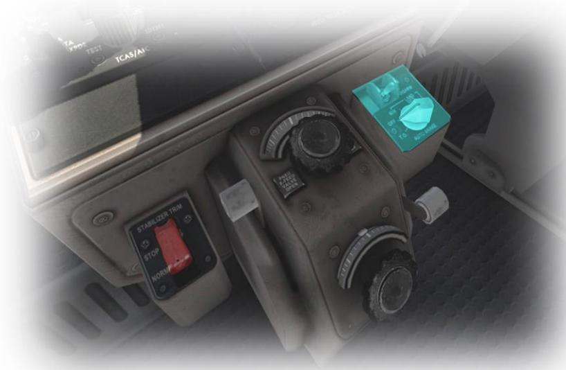
The Automatic Braking System applies brake pressure automatically during landing. This ensures the brakes are engaged at precisely the right time for optimum speed-reduction. This is particularly valuable when landing on a wet or snowy runway.
