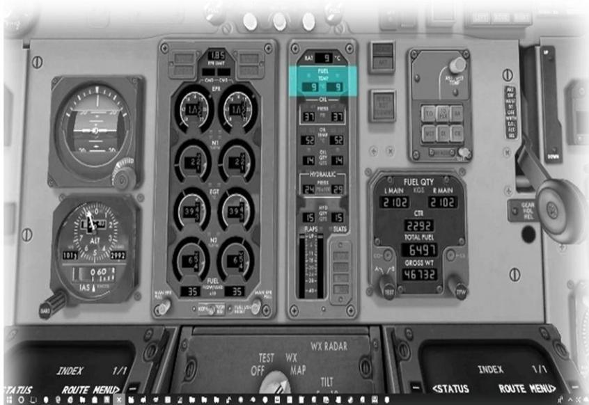
This is the temperature of the fuel, measured as it enters the engines.
