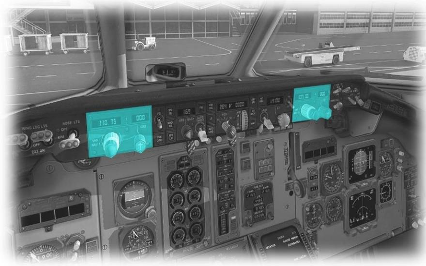
This aircraft is equipped with two VHF navigation radios (VHF NAV 1) and VHF 2.
