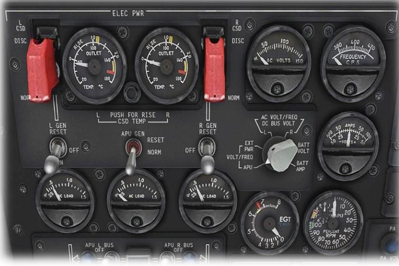
This panel is used to control and monitor the electrical power to the aircraft, when the main engines are running.
