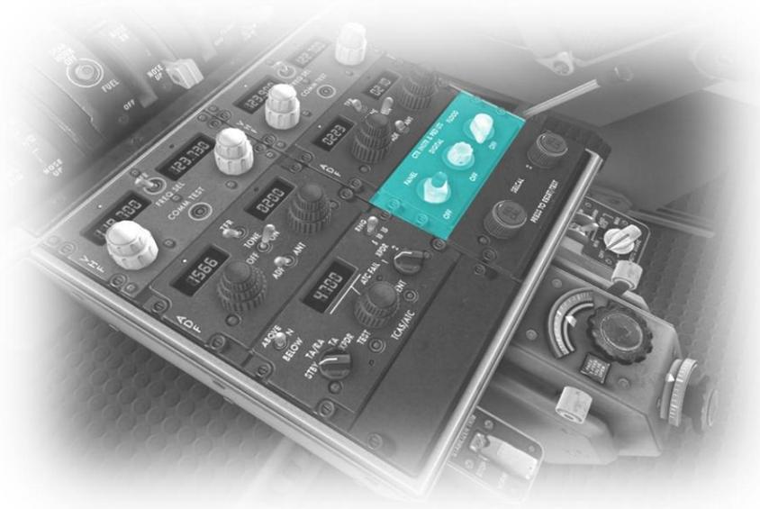
Use the 'PANEL' rotary control to adjust the back-lighting of the analog instruments contains in the Primary Instrument Panels.
