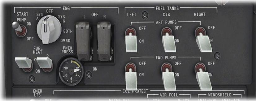
This panel controls the hydraulic pumps used for engine-start, and fuel flow (from the left, right and center tanks).
