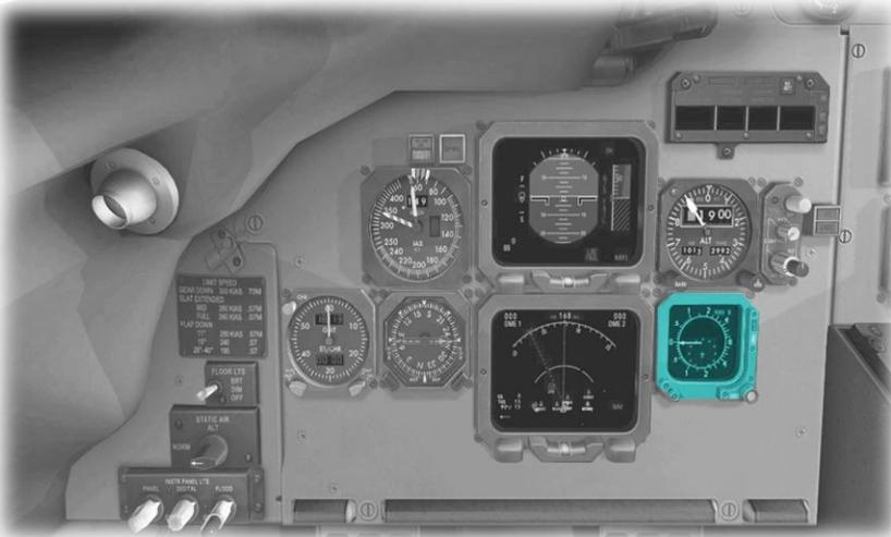
This instrument informs the pilot of the rate of climb, or the rate of descent, in terms of thousands of feet per minute.
