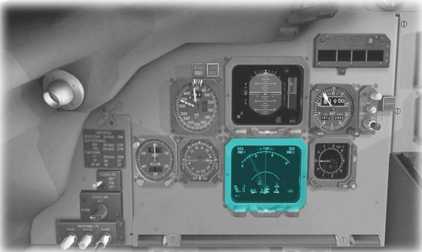
This is the lower LCD panel in the avionics cluster. The EHSI displays the aircraft's position & (magnetic) heading.
