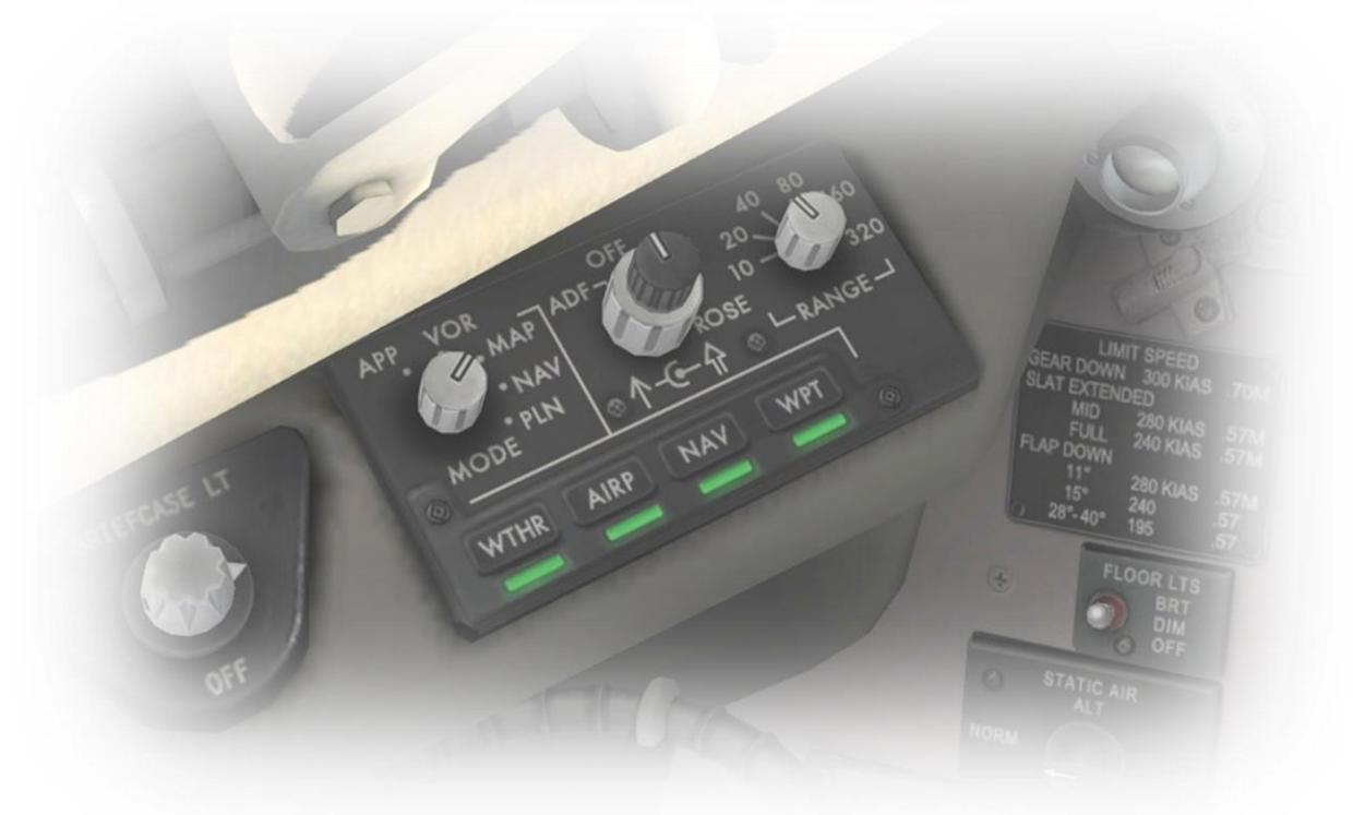
An EHSI Control Panel is provided for the pilot. This panel is used to customize the information presented on the associated EHSI display:
