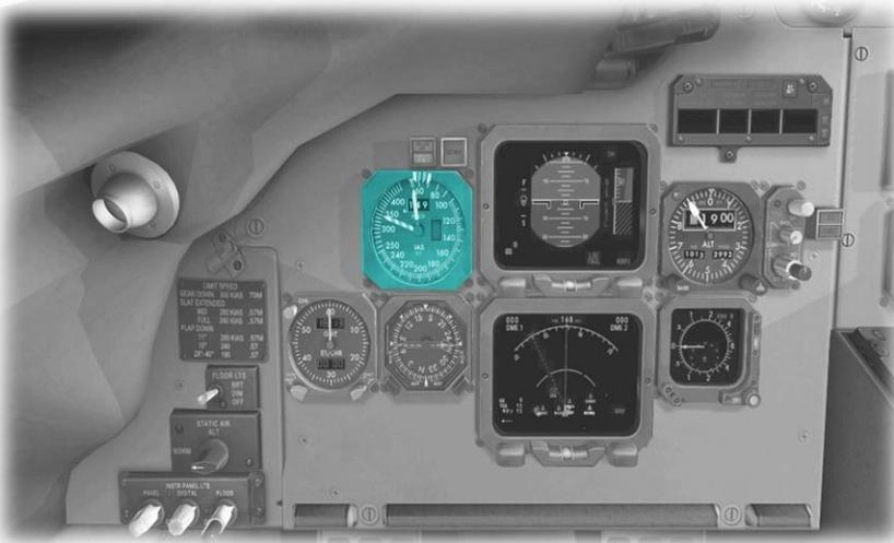
This instrument displays the speed of the aircraft (in knots) relative to the air (not the ground).
