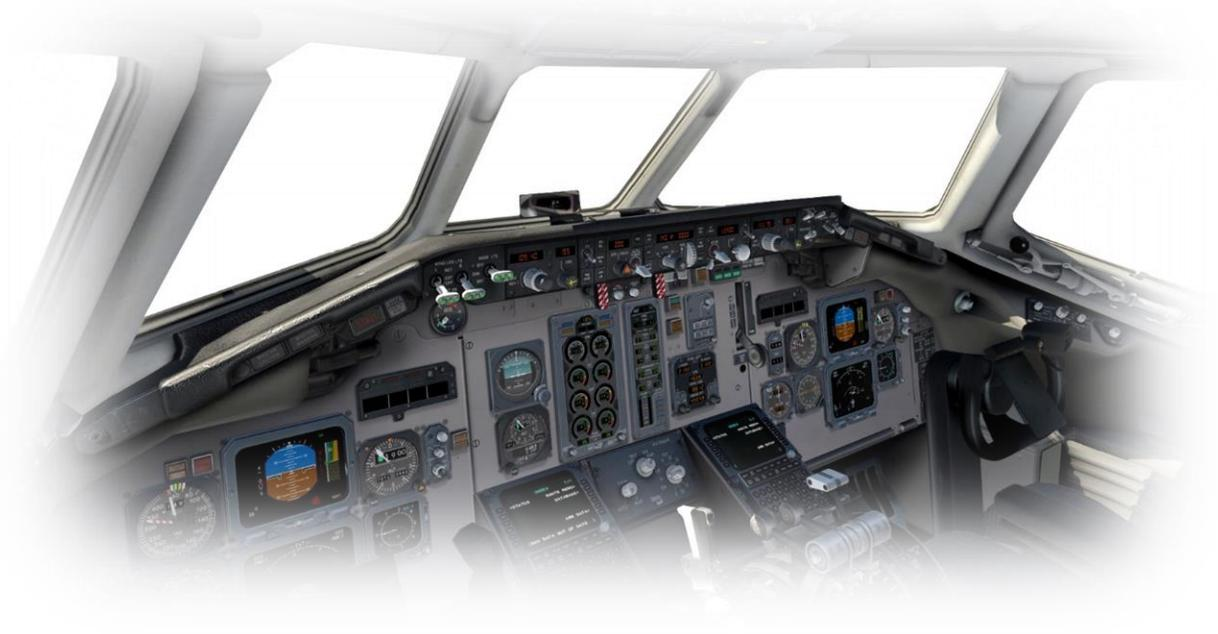
The X-Plane MD-82 features a detailed 3-D cockpit with a great many of the primary controls and systems modeled, including: Flight controls (yoke, rudder pedals, thrust levers, flap and speed-brake levers), electrical systems, pneumatic systems, navigation aids, radios, autopilot, interior and exterior lighting, and fuel systems.
