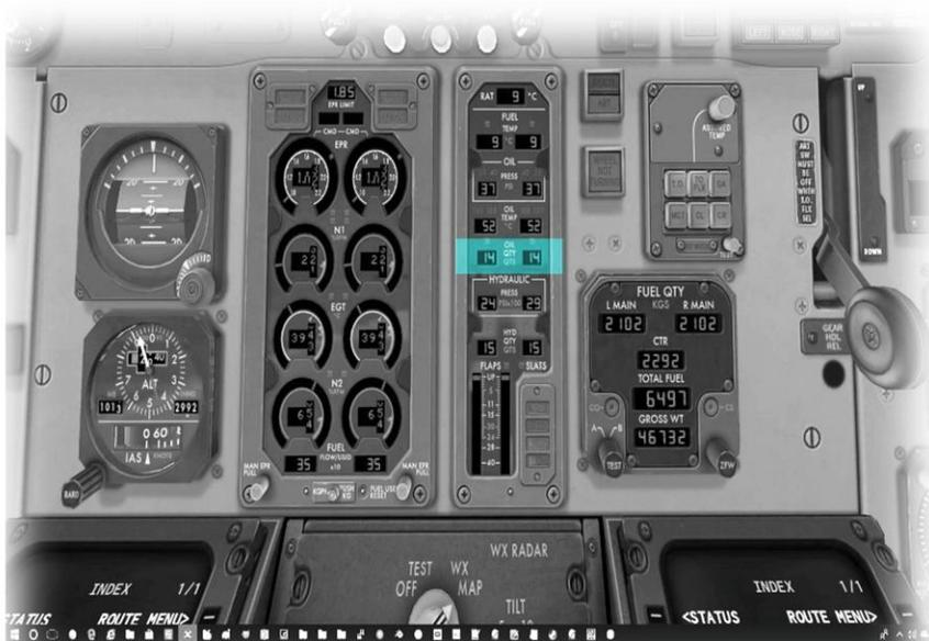
Left and right engine oil quantity respectively.
