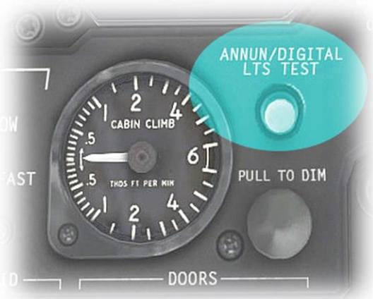
Note: A test switch is located on the overhead panel. Depressing this switch illuminates every light in the panel, to confirm each one is working.
