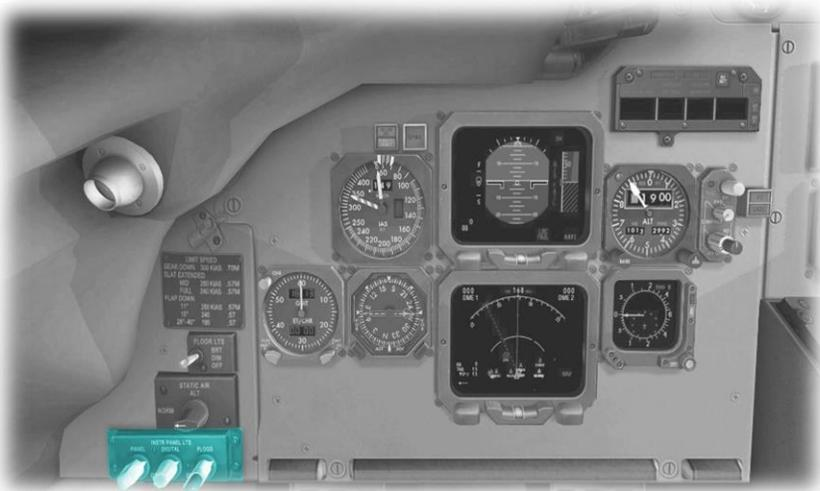
The rotary controls on this panel adjust (from left to right) the instrument back-lighting, digital display brightness, and overhead floods respectively.
