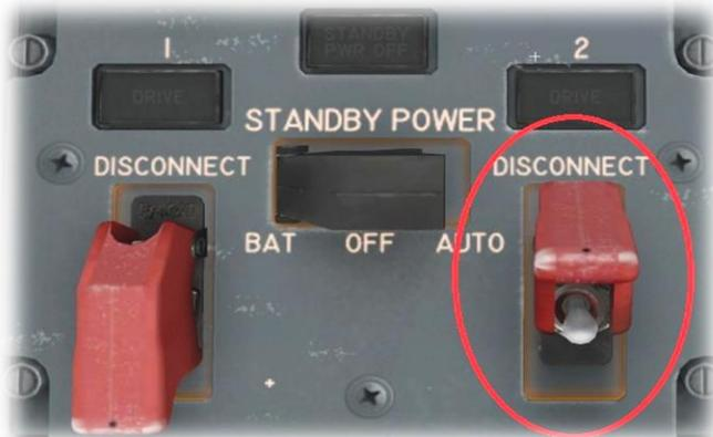
Guarded switches are used in situations where accidental activation of the switch must be prevented. To operate a guarded switch, the guard must first be opened. Do this by positioning the mouse pointer over the switch until the two vertical white arrows are displayed. Click once. If the switch is currently closed, it will open, and vice-versa. After the guard has been opened, the switch may be operated like a toggle and rocker switch (see earlier in this section).
