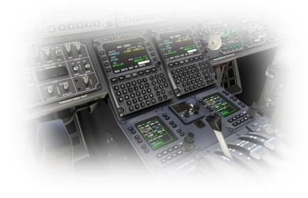
A Flight Management System (FMS) is a centralized computer system used in airliners, and other highperformance aircraft, to manage many of the aircraft systems, including (but not limited to) the flight plan.
