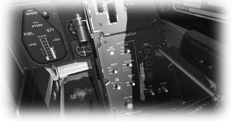
Fuel Quantity / Display Control Panel
